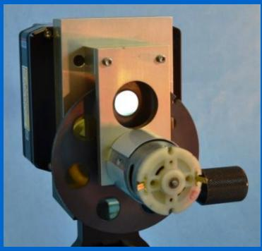
Line scan camera with 7 filters (H2O, Hydrocarbons)
